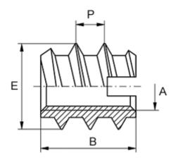
Female thread A = M14Length B = 26Male thread E = 22.0Min hole depth = 30
